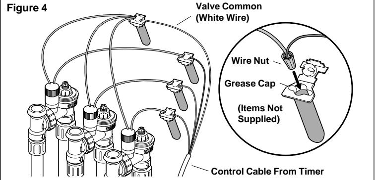
3. At timer, connect white common wire to the output terminal labeled "C" or "COM". Connect each color-coded valve wire to the numbered terminal in the order you wish the valves to operate during a watering cycle. Refer to the installation instructions furnished with the timer for additional information.
