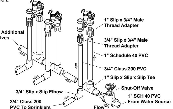
**Caution: Flush water supply line thoroughly before installing the valves! Sand and dirt in the line can damage the valve and/or prevent the valve from operating properly.**
